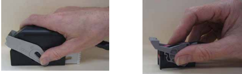
FIGURE 14. TYPICAL POSTURES USED TO POSITION MECHANICAL ASSIST CONNECTORS
