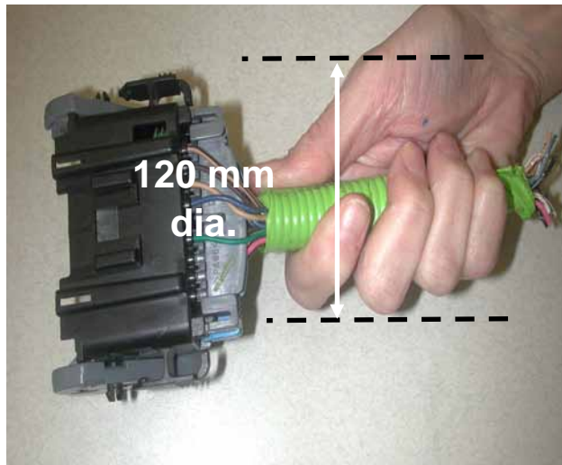
FIGURE 9. HAND GRASP CLEARANCE WITH BUNDLE
