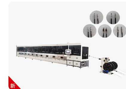
HBQ-910-H Automatic Processing Machine For Fakra Cable
